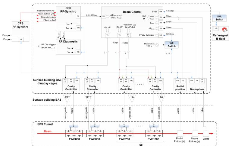
Figure 5 - SPS LLRF architecture
