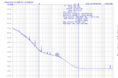
Figure 7 - recovered sampling clock from White-rabbit serial data stream
