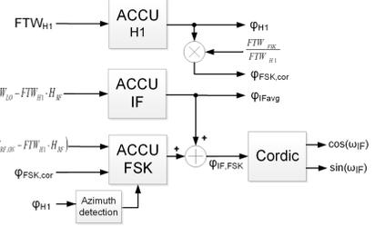
Figure 6 - NCO for up/down modulation in fixed frequency clock
