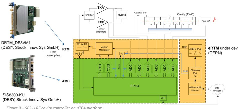
Figure 9 - SPS LLRF cavity controller on μTCA platform
