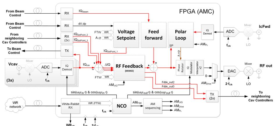
Figure 8 - SPS LLRF cavity controller diagram
