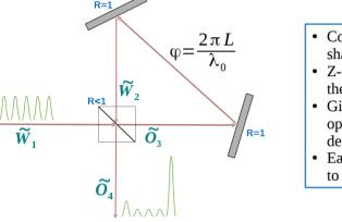
Consider the mirror as a digital filter, which shares the same transfer function. Z-transform is employed in algorithm for the implementation of FPGA. Give a direct link to the digital controller optimization, and also provides solutions to deterministic optical phase measurement. Easy to extend the system transfer function to cascaded cavities.
