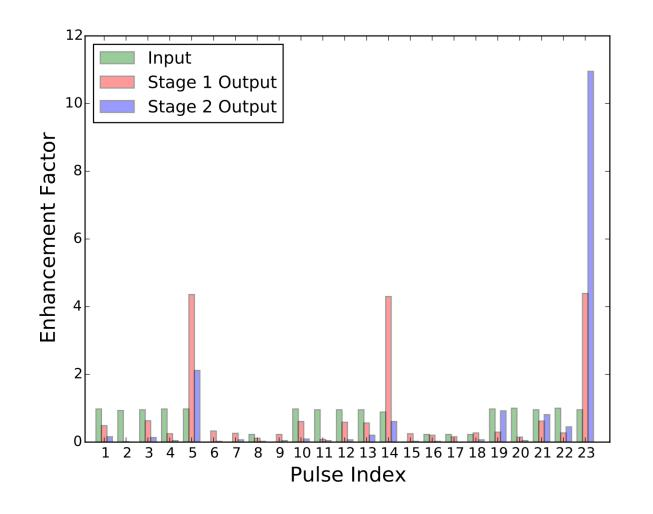
► A 2-stage (2+1 cavities) 15-pulse stacking system achieves a 11.0 peak-power enhancement factor, compared to the theoretical limit of 12.0.  $\blacktriangleright$  Each cavity is stabilized with 0.7° and 2.1° (RMS) phase errors for Stage 1 and Stage 2.  $10^{2}$ Stage 2 (Open Loop) Stage 1 (Open Loop) — Stage 2 (Closed Loop) Stage 1 (Closed Loop) 10  $(rad/\sqrt{Hz})$
