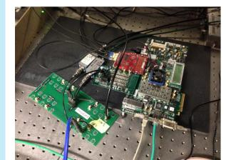
Hardware: ML605 + FMC110 + XM105 2-CH 12-bit A/D & 2-CH 16-bit D/A & 400Msps ► kHz Feedback Control Repetition Rate
