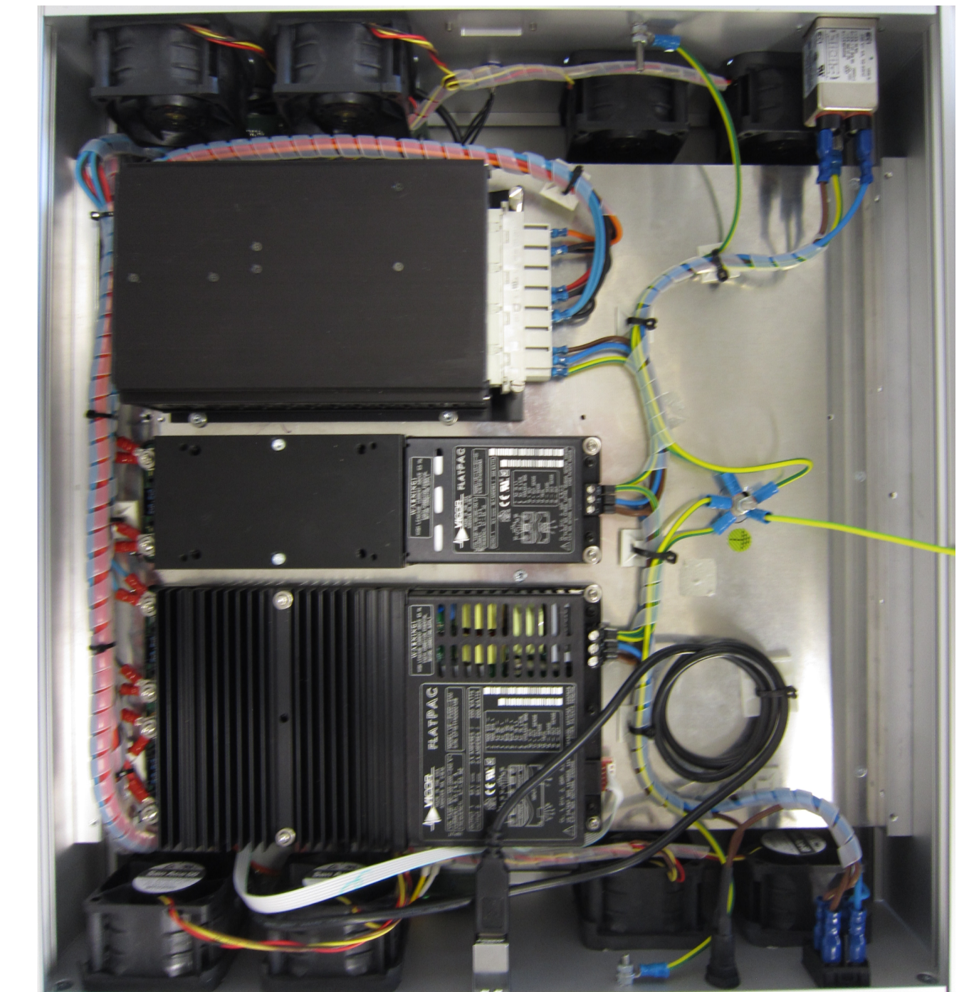
Piezo driver with package open. Upper – mainboard and PEM (PEM on the left side), bottom – power supplies
