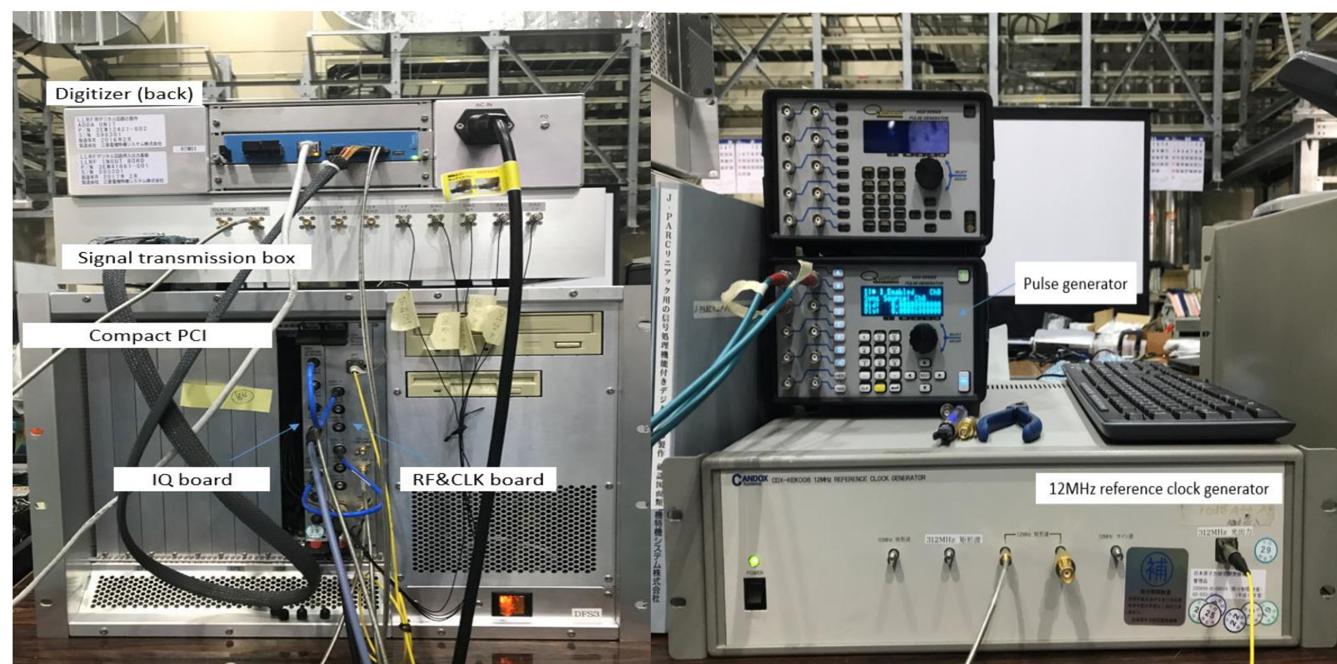
Fig 2. Low-level radio frequency control system
