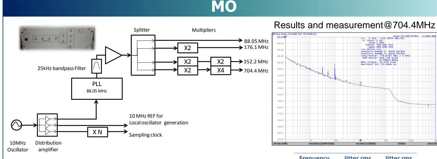
The Master Oscillator is realized using parts with Phase Noise requirements very hard providing by *ar Electronique* (OCXO, PLL) and Wenzel Associates (multipliers). A narrow bandpass filter allows reducing the PLL noise as it is shown on the plot.
