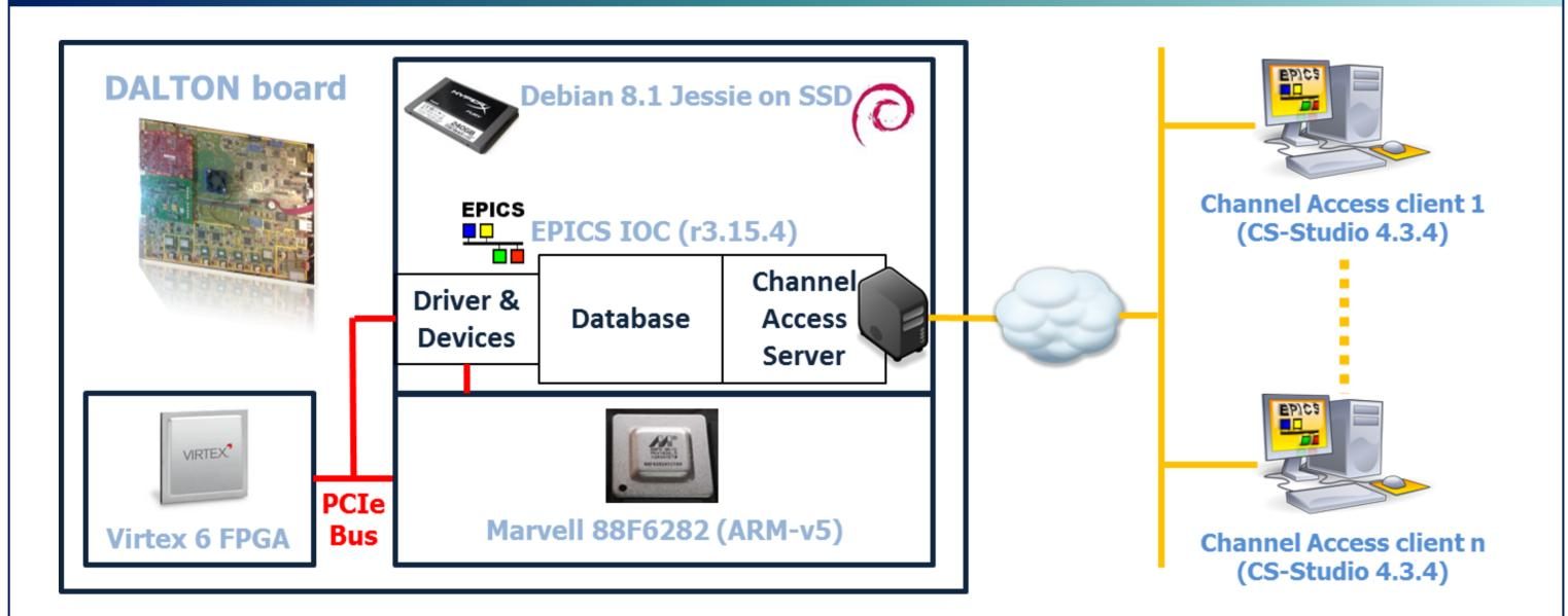
To perform the LLRF's control system, an EPICS I/O Controller (IOC) communicates with the FPGA. A PCIe bus drives data exchanges between the IOC and the hardware.
