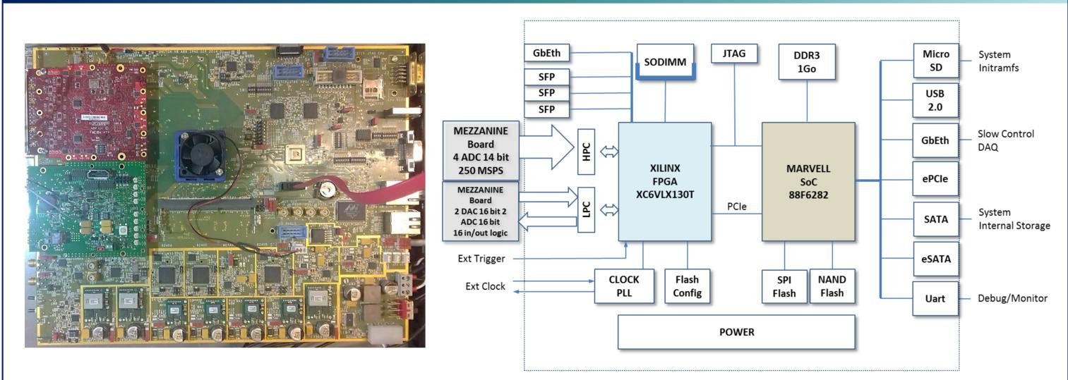
The DALTON motherboard board, developed at IPNO, is an in-house hardware solution to perform the control command and signal processing for the LLRF. It is equipped with a Xilinx Virtex 6 FPGA and a Marvell 88F6282 processor (ARM v-5 based), connected to each other with a PCIe bus.
