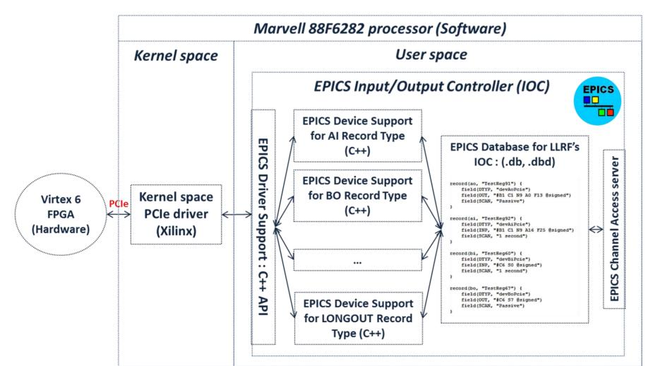
An in-house PCIe Linux kernel driver performs the communication with the FPGA. The driver layer of the IOC is a C++ API to wrap system calls and DMA and store hardware data. Then a device layer provides primitives to redirect inputs to the Process
