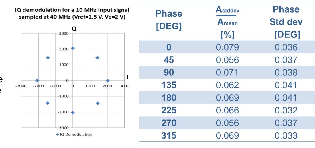
IQ Demodulation : ADCs tests with arbitrary functions generator AGF3102; better results are expected with the use of the master oscillator, see poster 54.
