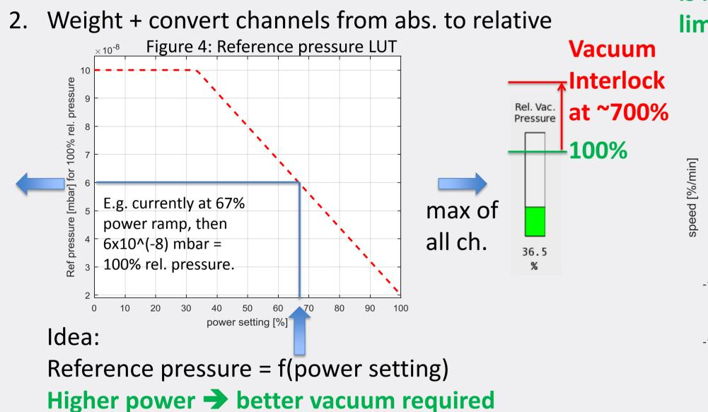
reading. Around 100 % rel. pressure the differential gain is 0 to get a stable operation point at the critical region. **Goal of the ramping speed control law** is NOT to reach the vacuum interlock
