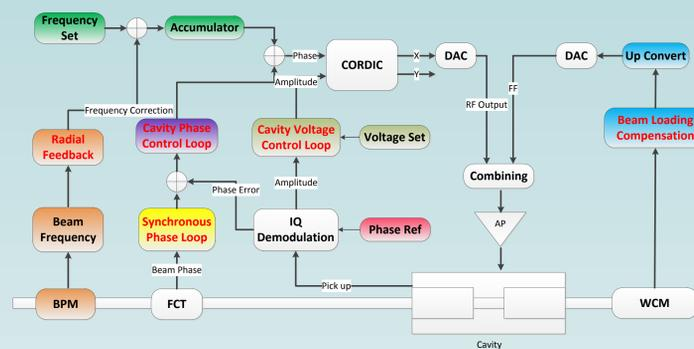
Figure.3 Reference Principle Diagram of the Multi-Control Loops
