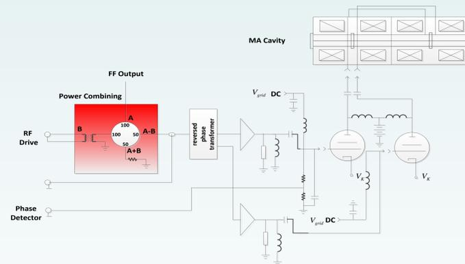
Figure.4 Schematic Diagram of Direct Feed-back Transmitter
