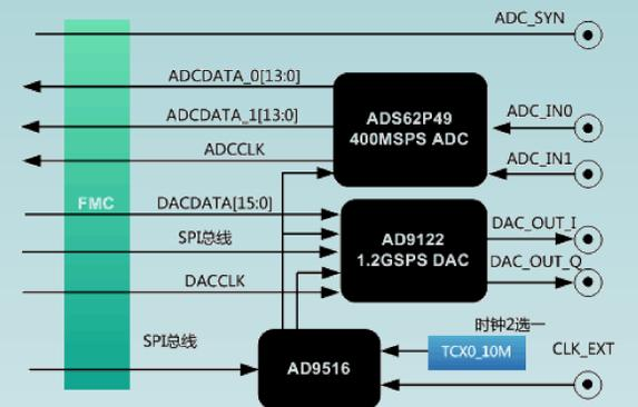
Figure.7 ADC/DAC Board Topology
