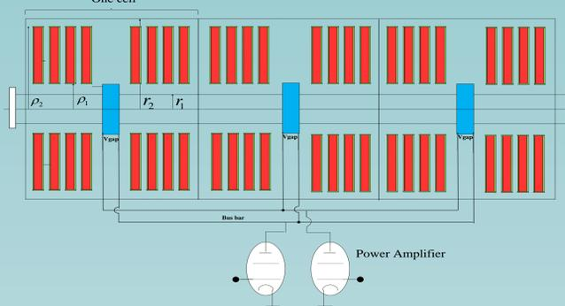
Figure.2 Structure of MA Loaded Cavity
