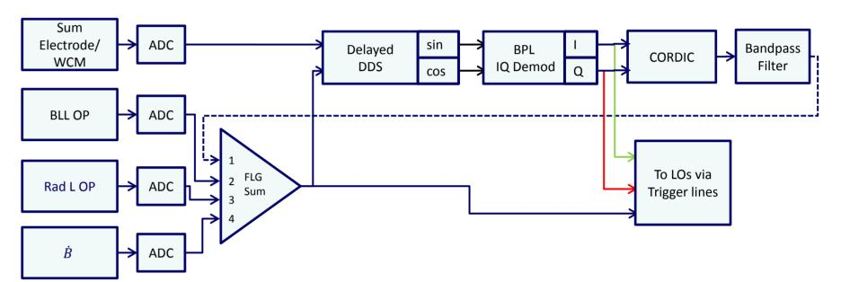
Previous used IQ tests demodulation of the beam sum electrode signal followed by a CORDIC algorithm to generate a beam phase signal. This will be implemented to replace the existing analogue beam phase loop with the added benefit of
