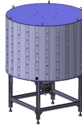
CERN 144:1 cavity combiner 144 kW CW @ 200 MHz calculations by ESRF within CRISP, construction by CERN
