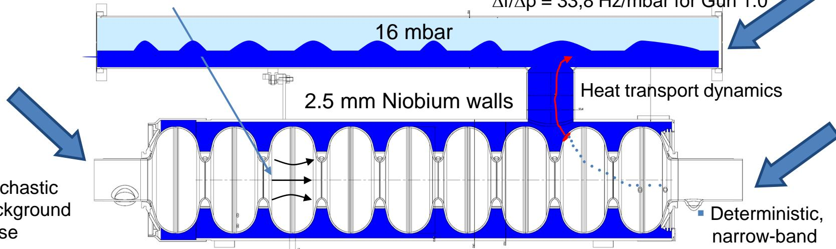
$$\Delta l = 1 \text{ nm} \leftrightarrow \Delta f = 0.6 \text{ Hz} \leftrightarrow \Delta \Phi = 1,14^\circ \text{ for BESSY-VSR Cav.}$$
