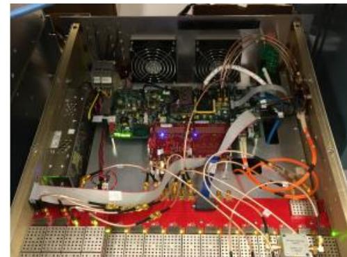
P-46 Digital Low Level RF control for Advanced Light Source
