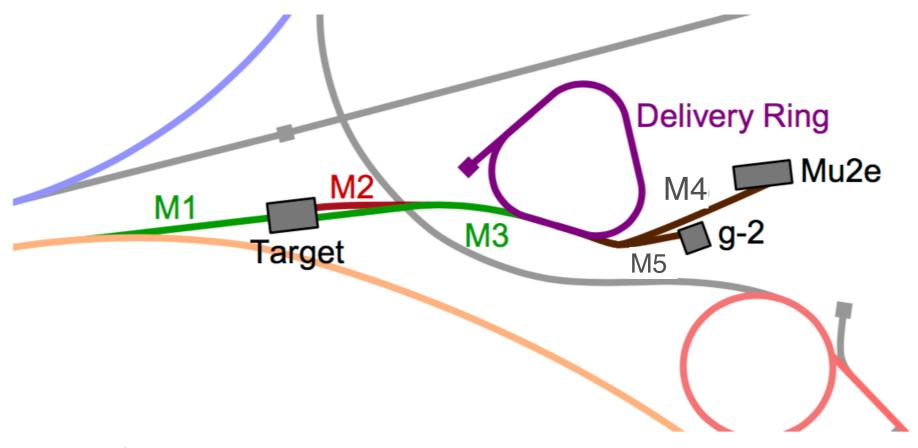
The Muon Campus consists of the Delivery ring, associated beamlines, the target, the g-2 experiment, and the Mu2e experiment. The five beamlines, designated M1 through M5, direct beam to the Delivery ring and from the ring to the experiments. The path that the beam takes through the Muon campus depends on which experiment is taking beam. For this reason, only one experiment is run at a time.
