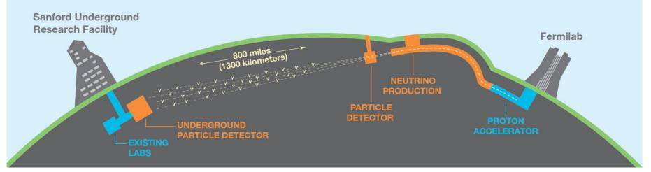
The Deep Underground Neutrino Experiment (DUNE) is a leading-edge, international experiment for neutrino science and proton decay studies. DUNE will consist of two neutrino detectors. One detector will record particle interactions near the source of the beam, at Fermilab. A second, much larger, detector will be installed more than a kilometer underground at the Sanford Underground Research Laboratory in Lead, South Dakota — 1,300 kilometers downstream of the source.
