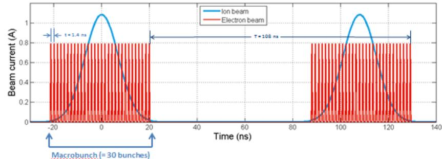
Electron bunches are generated in the DC gun with a repetition rate of 704 MHz. Macrobunches (consisting of ~30 bunches) repeat at the 9 MHz ion bunching frequency. These frequencies are both harmonics of the RHIC ion revolution frequency, but the 704 MHz harmonic is not an integer multiple of the 9 MHz harmonic.
