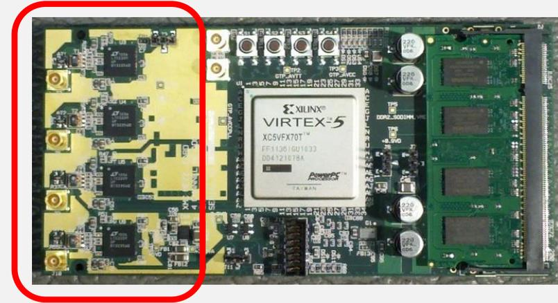
Platform XMC 4CH High Speed ADC Board
