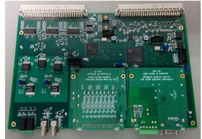
Carrier card w/ 8 CH RF Detector & Interface FMC
