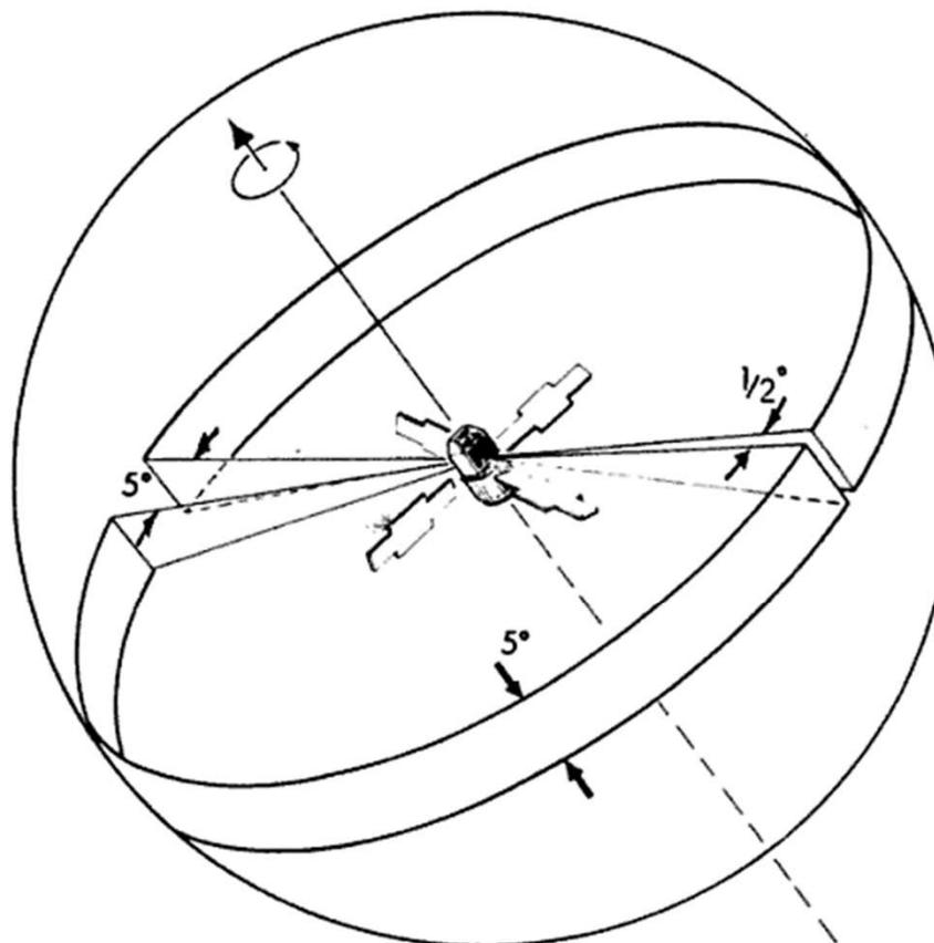
5. Scan geometry of the UHURU X-ray detectors shown as the projection on a sphere. As the satellite rotates the X-ray detectors view in a 5° band, 90° from the spin axis.
