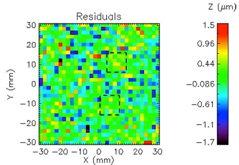
*Test using Corning Eagle™ flat glass, 0.4 mm thick, 100 mm diam., 1 cm<sup>2</sup> piezo cells*
