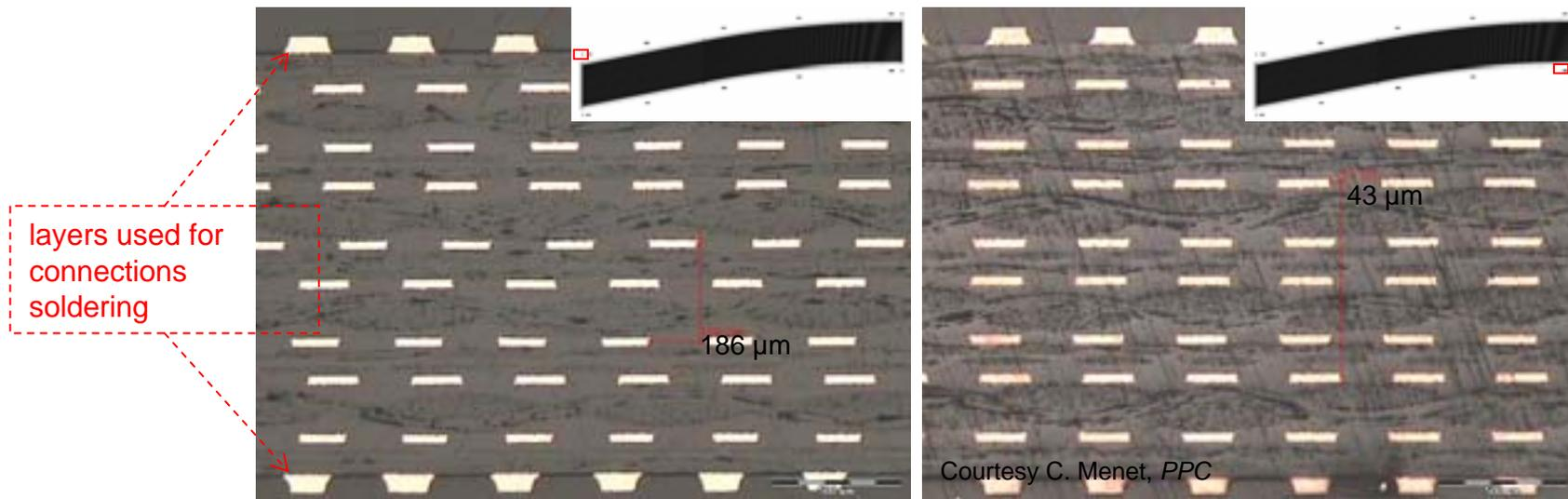
Maximum misalignment (longitudinal) Minimum misalignment (horizontal)
