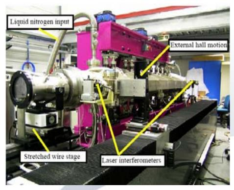
J.Chavanne, M. Hahn, R.Kersevan, C.Kitegi, C.Penel, F.Revol, Construction of a cryogenic permanent magnetundulator at the ESRF, EPAC'08 Proceed., p. 2243. Spring-8 (SAFALI)
