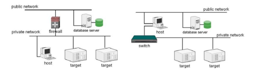
A configuration where host and targets are in the same protected subnet accessed via a firewall. A configuration where host has two NICs and accesses its instrumentation on a private LAN.
