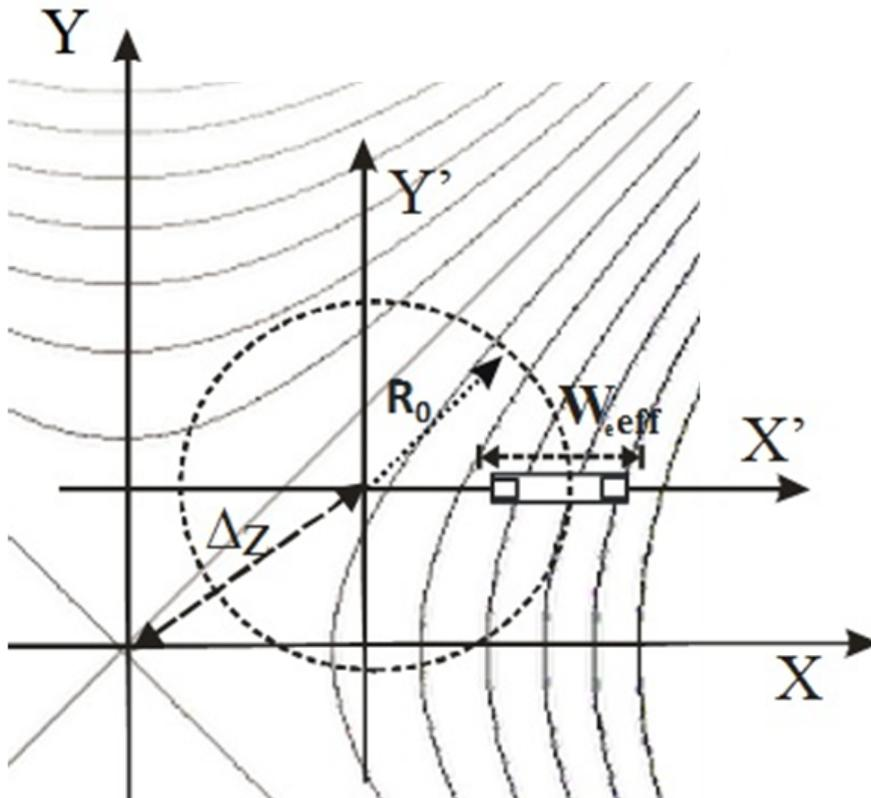
Radius ( $R_0$ ) and surface ( $A_c$ ) of the coil have to be determined: 2 unknowns
