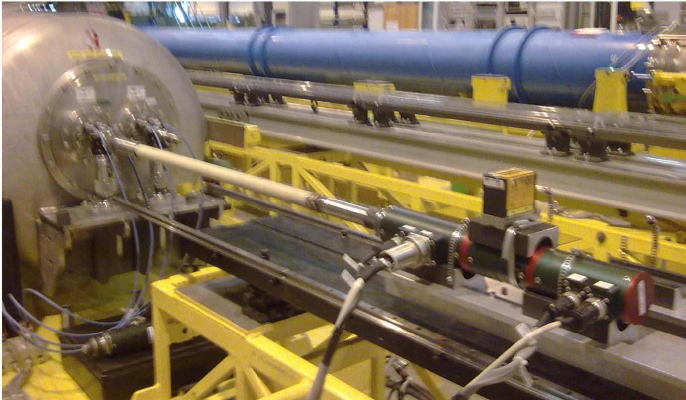
Shaft composed by 12 segments of 1150 mm mechanically connected in series
