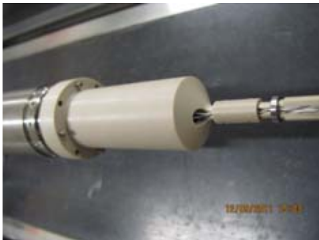
Connection of the shaft to the MRU motor unit
