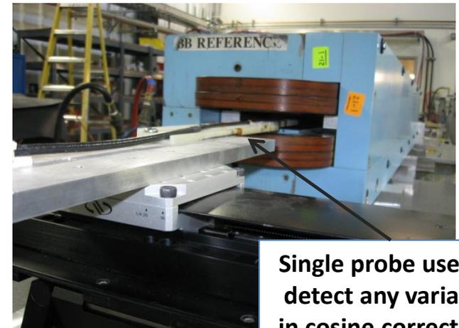
Single probe used to detect any variance in cosine corrections for trolley probes
