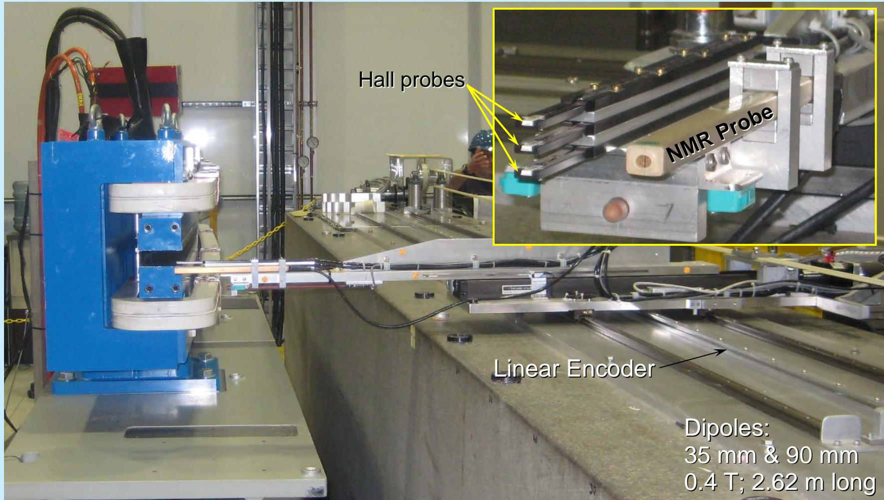
4.28 m axial travel; 0.33 m radial travel; 5 micron resolution position readout
