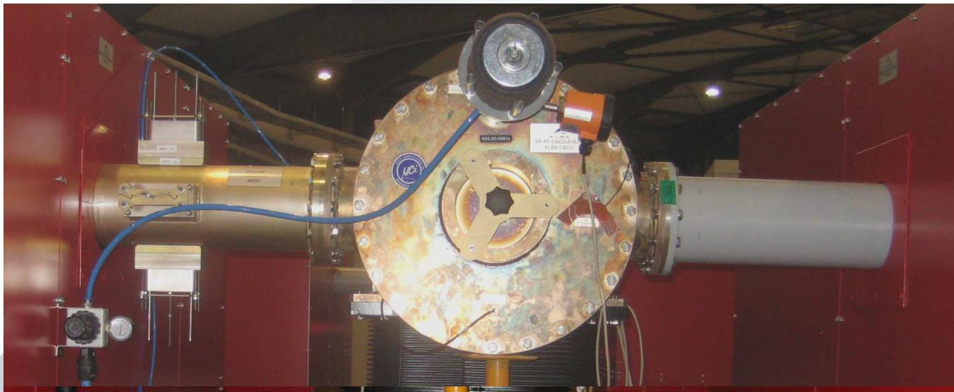
With CoStubs, if one IOT is not operational, we still can power that cavity with only one IOT
