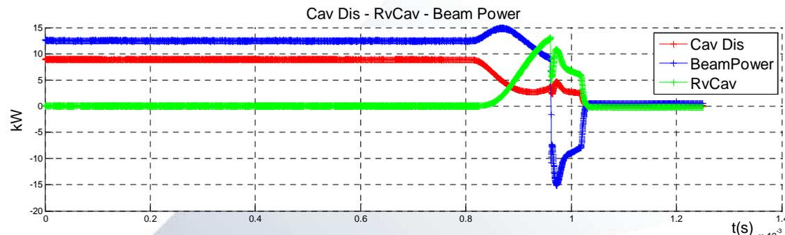
**Provisional solution: Reflected power interlock level increased up to 23kW**
